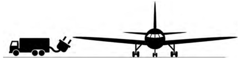
Figure 39. Electric aircraft charging via a mobile supercharger.
