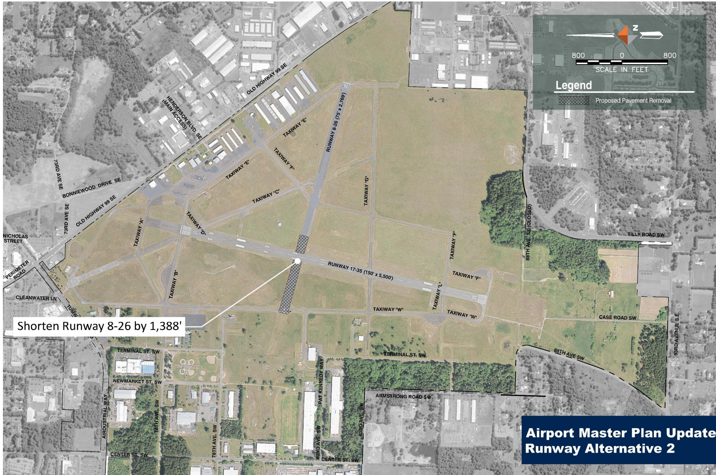
Figure 4-5: Runway Alternative 2 Layout
